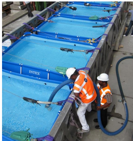
Figure 10: For the testing of the bridge, water containers were filled with water
